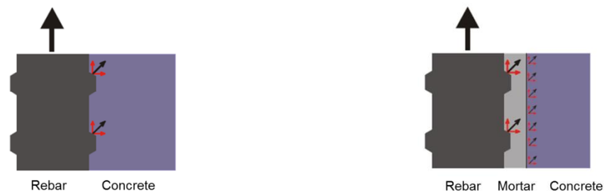
Figure 27 – Load transfer mechanism of a cast-in rebar and a post-installed rebar, schematically
