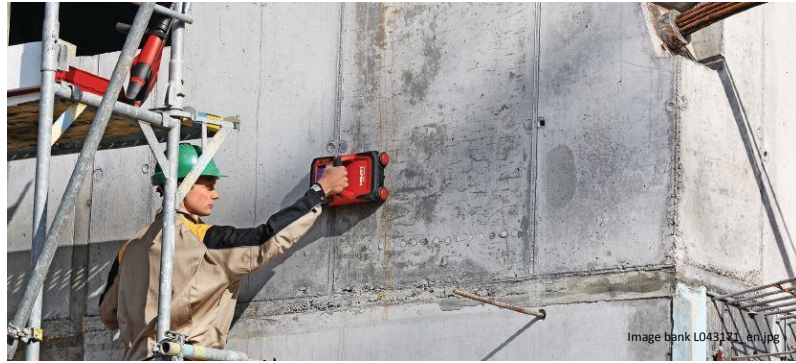
Figure 4– Scanning for reinforcing bars and other embedded items with a Hilti GPR scanner.
