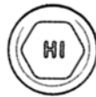
FIGURE 4—DEPICTION OF IDENTIFYING MARKING “HI” FOR HILTI S-BT SCREW-IN STAINLESS STEEL FASTENERS,
